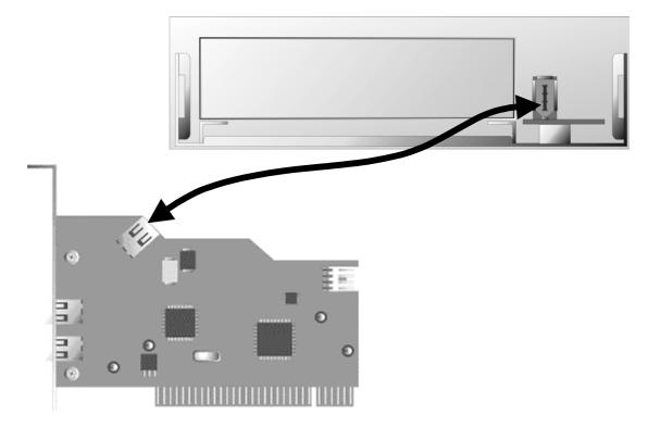
If you wish to connect IEEE-1394 devices, that do not have an independent power supply, we recommend you to connect the computer's power supply to the Cameo Connect. This avoids an overload caused by extensive power consumption of IEEE-1394 devices
