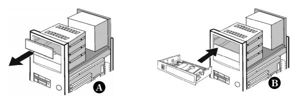
Attach the front module to the computer's enclosure, using the included screws.
