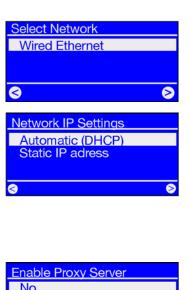
1) If a wired connection is available, then "Wired Ethernet" is the correct choice.
