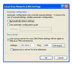
Open Internet Explorer, select "Internet Options" from the "Tools" menu and select the "Connections" tab. On the bottom third of the tab, you'll find the "LAN Settings..." button. Press the button to open the dialog box shown here.
