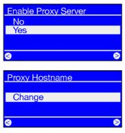
1-3) To set up the NOXON to work with a proxy server, follow steps 1 & 2 as described above... and in step 3 (Enable Proxy Server Yes/No), select YES!
