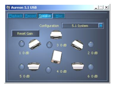
Under each speaker is a label. The first digit (1-6) indicates the output jack of the Aureon 5.1 USB to which that speaker should be connected. The other part of the display (+/- 20 dB) is a readout of the volume dials which are next to each speaker.
