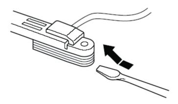
The double-sided adhesive can be rolled off the underside of the pickup with a fingertip. Correct the height of the pickup by adding or removing spacers.
