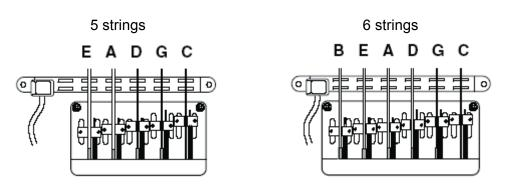
Each string must be positioned over its magnet pair.
