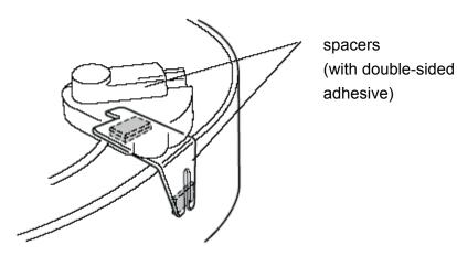
As an elegant alternative, you can also attach the bracket to the instrument with the strap button (using spacers if possible to avoid scratches). Loosen the strap button of the instrument by unscrewing it a couple of turns and insert the slot of the bracket under the button. Tighten the screw to secure the bracket to the body.
