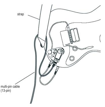
To unplug the 13-pin cable from the AXON or the AIX 101/103, press the unlock button on the plug body.
