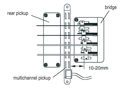
The pickup is suitable for bass guitars with up to six strings (6B, 5E, 4A, 3D, 2G, 1C). In the case of four-string basses, the four central magnet pairs must be positioned under the strings, leaving one pair at either end of the pickup unused. The mounting position for five-string basses depends on the tuning: for [B, E, A, D, G], the magnet pair opposite the cable end, for [E, A, D, G, C] the magnet pair at the cable end is unused, as shown below.
