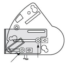
Apply two spacers (with double-sided adhesive) to the bracket to prevent scratching the instrument's finish and attach the controller to the instrument as shown.
