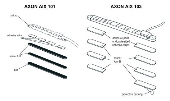
**Note:** the reusable adhesive pads may be used as the bottom (guitar-side) layer. Trim the pads as required to match the shape of the pickup.
