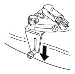
**CAUTION!** The screw of the strap button can loosen due to repeated removal and tightening or strong pressure on the bracket.
