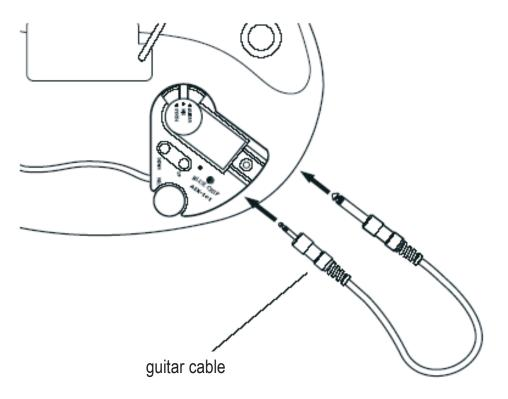
**Note:** connect the instrument cable even if you will not be using the conventional pickup sound. This connection is important for grounding the instrument to prevent noise and electric shock.
