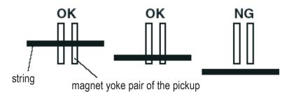
Once the pickup is correctly aligned, mark the centers of the screw holes with a sharp pencil or punch on the bass top. If you do not want traces of the marking to remain on the top, use small pieces of marking tape instead of a pencil.
